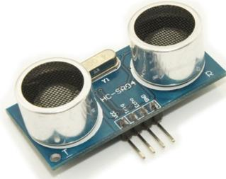
The interface to the KSR504 features 4 connections. +5V power, Send Control, Received Signal Out and Ground.
