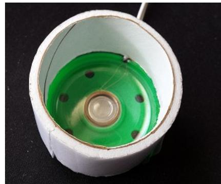
**Trick 2.** A Cardboard Speaker Enclosure. In fact, just about any box that can hold the speaker would do. Even as small as a matchbox. Yes!! It takes a bit of care and some nibbling at the box so that the speaker frame just peeps through the box's sides but it can be done.
