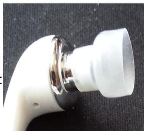
When this is fitted snugly over the electret microphone like this, it gives us great acoustic coupling and effectively shuts out unwanted ambient noise.
