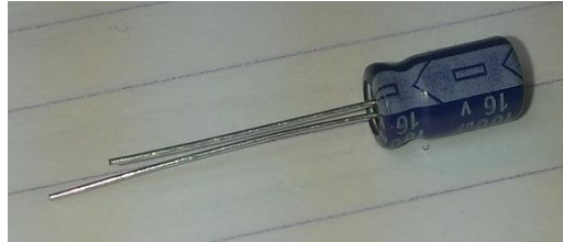
Fig 6.2 Showing the different leg lengths and the “-“ marking on the body of an electrolytic Capacitor.
