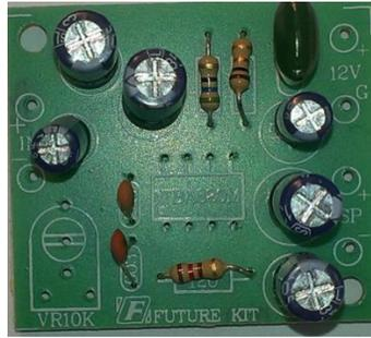
Fig 5.6 Showing the PCB with all six of the electrolytic Capacitors installed.
