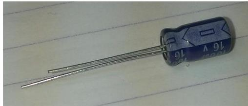
Fig 5.4 Showing the different leg lengths and the “-” marking on the body of an electrolytic Capacitor.
