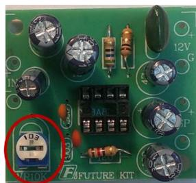
Fig 7.1 Showing the trimpot installed.
