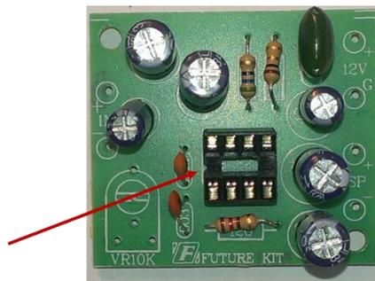
Fig 6.1 Showing the PCB with the IC Socket installed, and the “notch” highlighted for correct orientation.
