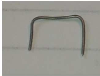
Fig 3.4 Study of the “Jumper” which we made from the cut off leg of a resistor. (Shown larger than real-life size).
