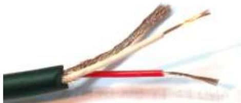
*Fig 6: Audio cable with all three conductors ready for tinning.*
