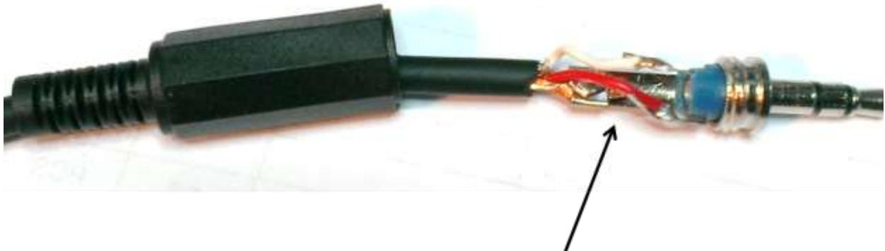
Study showing the internal connections for the 3.5mm plug.
