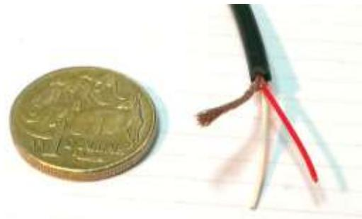
*Fig 5: Audio cable with shield carefully gathered together before stripping the centre conductors.*
